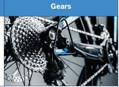
A gear is also known as a cog. They are like wheels but have 'teeth'. A gear or set of gears can be used to change the speed or direction of a force. If one gear turns clockwise then the other will turn anti-clockwise.
